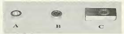
FIGURE 1: Mini-mesocosms in aluminium stubs of 4 mm height and 10 mm diameter. The cavities are 3 mm in depth and 6 mm in diameter (A). Small aliquots of thoroughly homogenized sediment samples are transferred into the cavities of aluminium stubs (B). These can be placed in humid chambers under defined conditions of e.g. light, temperature and salinity. After cryofixation, the stubs are mounted onto a specimen holder (C) and transferred into cryochamber attached to a scanning electron microscope.
